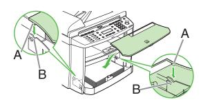
Connect the edge of dust cover (A) and the edge of paper cassette (B).
